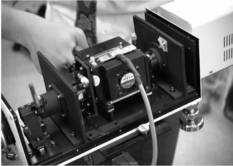
Figure 3: Interior photograph of the camera's spectroscopic section
