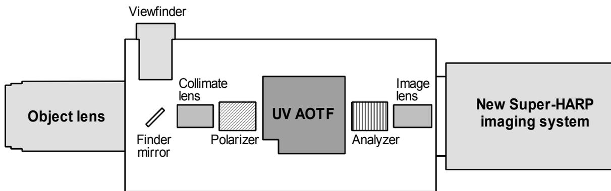
Figure 2: Conception diagram of UV and visible hyperspectral camera
