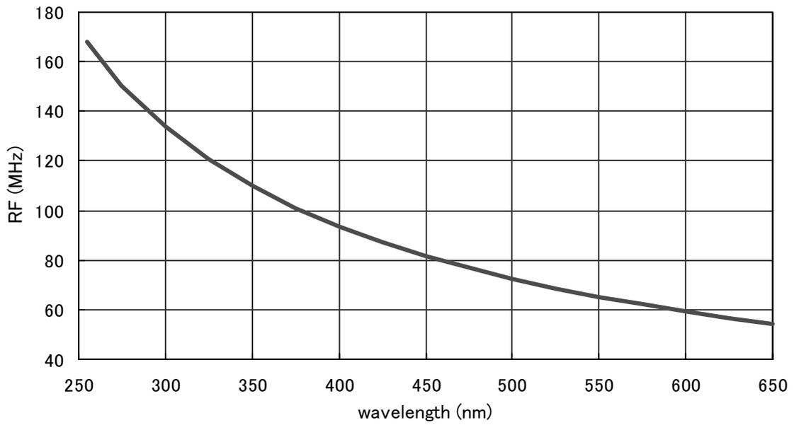
Figure 5: Tuning characteristic of filter light wavelength versus applied acoustic RF signal
