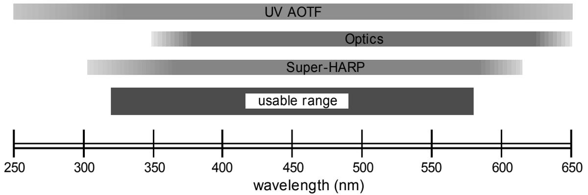
Figure 7: Spectral range of UV and visible hyperspectral camera
