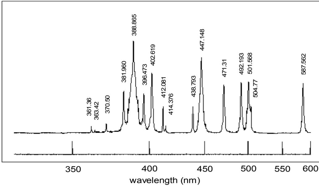
Figure 6: Spectral analysis for helium-discharge lamp light
