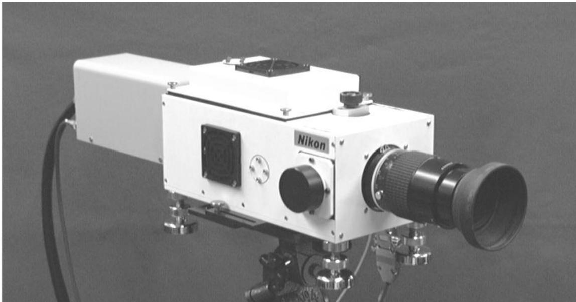
Figure 4: Appearance photograph of the UV and visible hyperspectral camera
