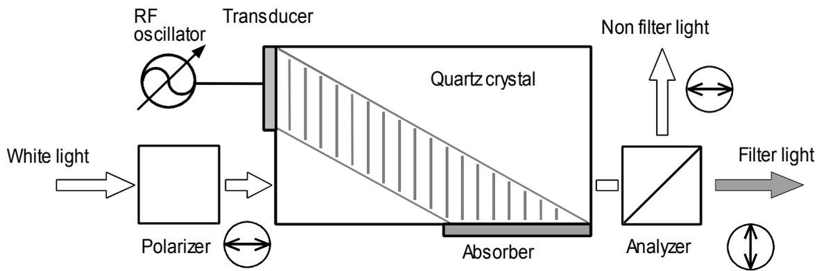
Figure 1: Principle of collinear AOTF
