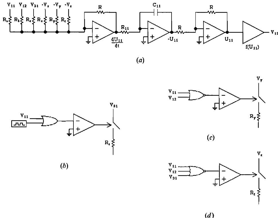
**Figure 8.** Circuit diagram of the 11th processing element in Fig. 7: (a) analogue circuit diagram of the 11th processing element; (b) circuit for the omega function heuristic ( $B$ -term); (c) circuit for the hill climbing heuristic ( $C$ -term); (d) circuit for the hill climbing heuristic ( $D$ -term).
