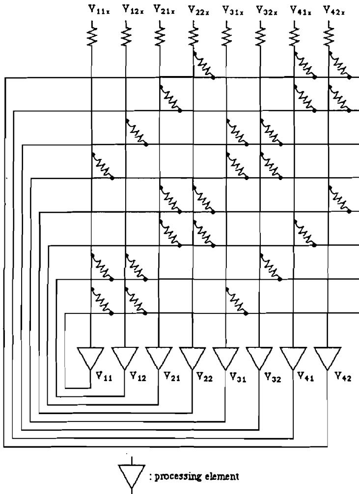
Figure 7. Circuit diagram of the neural network for the 4-vertex 4-edge graph problem in Fig. 6.
